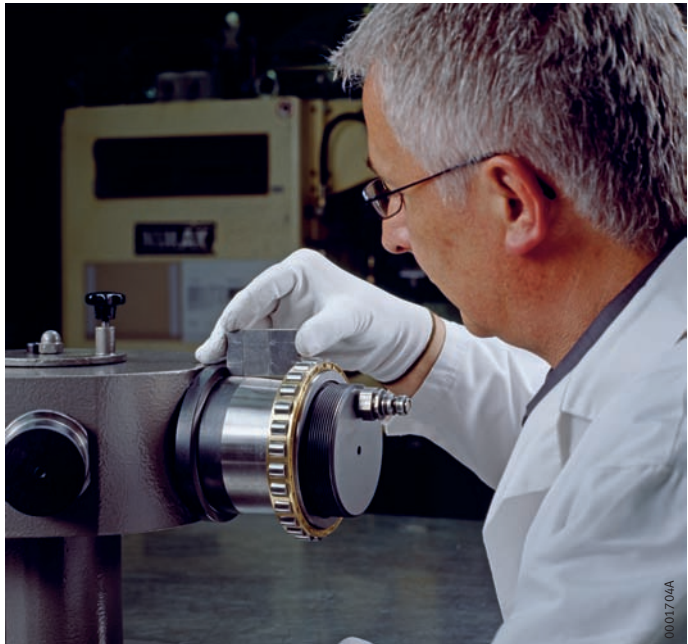
Figure 5 Measuring the distance to the shaft shoulder
