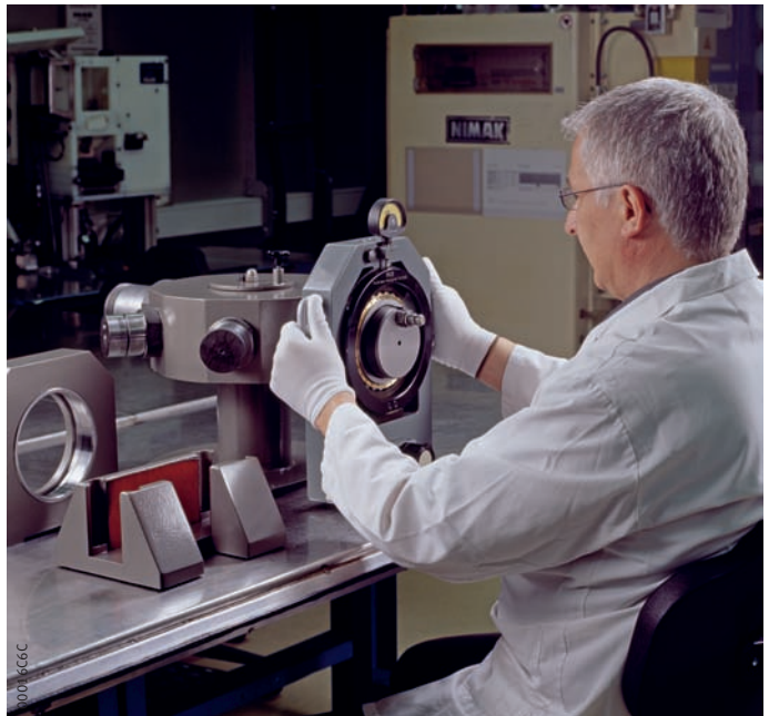
Figure 4 Positioning the enveloping circle gauge
